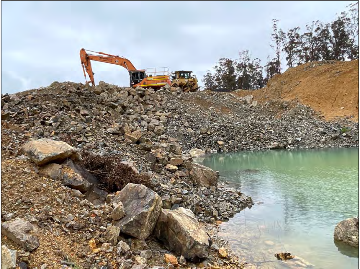
Figure 10: Central part of the existing quarry, high to very high strength meta siltstone.
